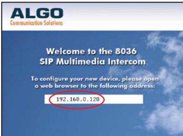
3. Note the IP address displayed and enter this into your PC's web browser to display the 8036 Control Panel. Login with the default password ("algo").
